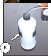
Periodically replace the cooling lubricant that is contained in the relevant tank (B). failure to observe this rule will invariably cause machining to be rougher and the mills to wear out more rapidly In the event that increased tool lubrication is required, use the regulator (C) of the exit of the cooling soupape which is placed inside of the machine near the blade.
