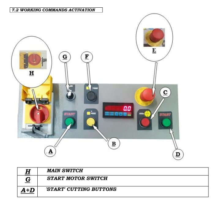
After the clamps are closed and the main switch (H) is activated, it will be possible to start the blade motor turning the switch (G). Press both the (A+D) buttons to start cutting. The protection cover will close and the blade will start rising.
