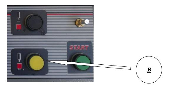
It is necessary to close the protection cover then the clamps must be closed otherwise the blade motor will not run.
