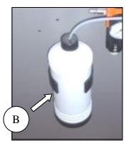
Periodically replace the cooling lubricant that is contained in the relevant tank (B). failure to observe this rule will invariably cause machining to be rougher and the mills to wear out more rapidly In the event that increased tool lubrication is required, use the regulator (C) of the exit of the cooling soupape which is placed inside of the machine near the blade.
