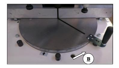
To cut at intermediate angles just leave the table in the intermediate position then turn the lever (A) in the arrow direction.
