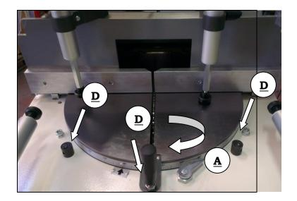
If the machine does not cut properly in one of the preimposted angles  $(0^{\circ}/45^{\circ})$ , regulate with a key the locking eccentric pin (D) till the cut will be the most accurate.
