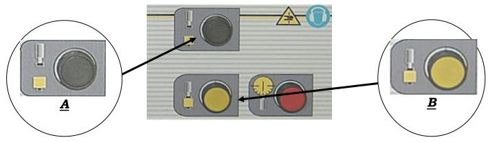
To close the clamps press (B) button. When the working phase is finished press (A) button to open the clamps unlocking the worked profile.
