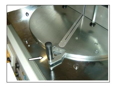
If the machine does not cut properly in one of the imposted angles (0°/45°/-45°), regulate with a key the locking eccentric pin (D) till the cut will be the most accurate.
