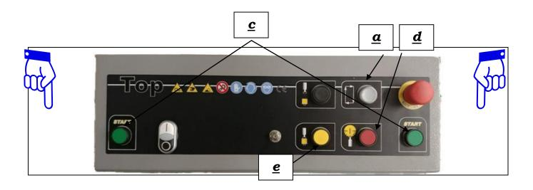
Press at the same time both (c) buttons to close the protection cover and start the blade rising. Once finished release both the buttons to permit the descending of the blade.
