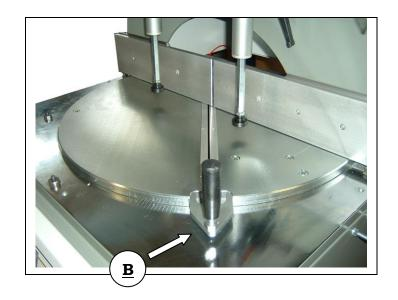
To cut at intermediate angles just leave the table in the intermediate position then release the locking button.
