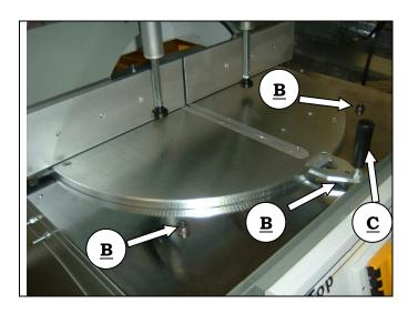
Rotate the table till it is positioned to the **45°reference (B)** if you need a 45° cutting.
