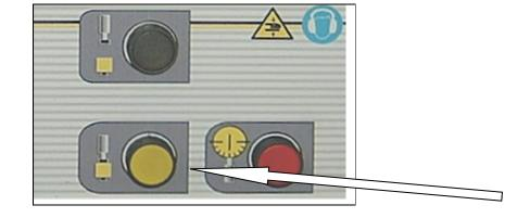
It is necessary to close the clamps otherwise the blade motor will not run. To close the clamps the CLAMPS CLOSING BUTTON (B) must be pressed.
