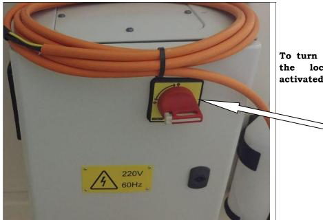
To turn on the cutting off machine the lockable switch must be activated (A).
