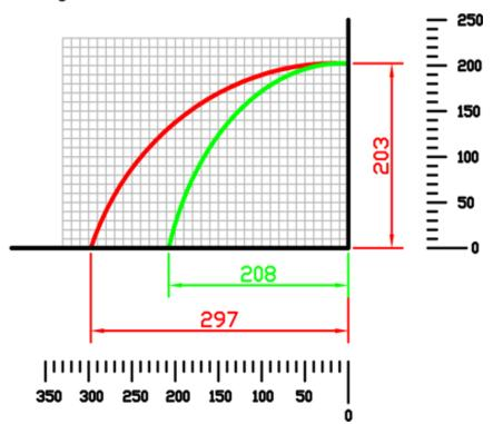
DIAGRAMMA DI TAGLIO TRONCATRICE ASCENDENTE TOP CON LAMA Ø600mm CON SQUADRO SPOSTATO DI 200mm
