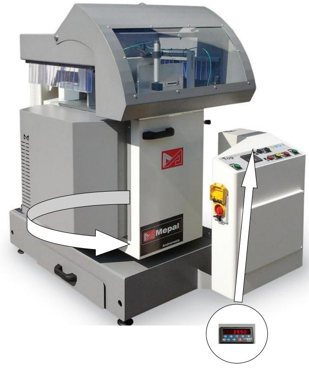
The angle displayed on the screen is calibrated placing the head at  $90^{\circ}$ .
