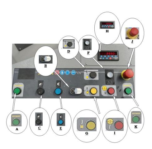
It is necessary to close the clamps otherwise the blade will not rise. To close the clamps the CLAMPS CLOSING BUTTON (G) must be pressed.
