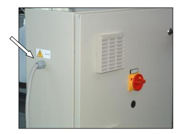
**ATTENTION**: if a chips belt conveyor is installed on the machine, once the connection to the electrical line and a suitable grounding are made it is necessary to verify the correct motor rotation: looking at the machine from the front side, the chips belt conveyor must turn clockwise.
