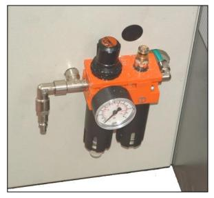
The machine control system pressure is made with the pressure regulator control knob: clockwise to increase and counterclockwise to decrease. The lowering of pressure takes place through the adjustment relieving of the regulator and, therefore, it is advisable to flow over the predetermined value, wait a few seconds for the stabilization and then go up slowly.
