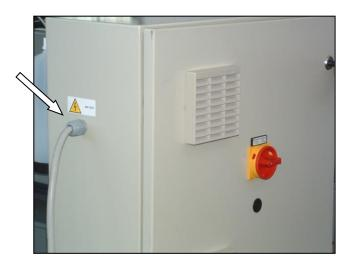
**ATTENTION**: Made the connection to the electrical line and a suitable grounding it is necessary to verify the correct motors rotation: if the blades are fixed to the crankshaft nut agree with the direction of rotation. Reversal of rotation, with even a limited duration, could cause the unscrewing by inertia, with dangerous consequences. Adhere to the following:
