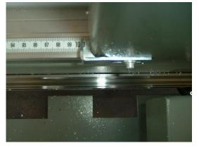
A graduated rod is installed in front part of the basement for reading of the blades' wheel-base.
