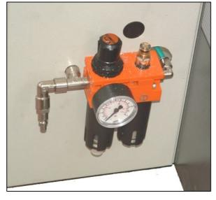
The machine control system pressure (6 bar) is made with the pressure regulator control knob: clockwise to increase and counterclockwise to decrease. The lowering of pressure takes place through the adjustment relieving of the regulator and, therefore, it is advisable to flow over the predetermined value, wait a few seconds for the stabilization and then go up slowly.
