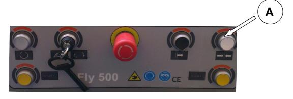
While the clamps are closing, if the hands of the operator stay blocked between the clamp and the profile or between the profile and the surface plate, the starting of the machine is performed at low pressure (about 1 bar), in such a way to avoid crushing danger. During the cutting phase, when the operator has both hands engaged and away from the work piece, the pressure switches to the value of the mains, reaching the maximum force of bracketing the work piece.
