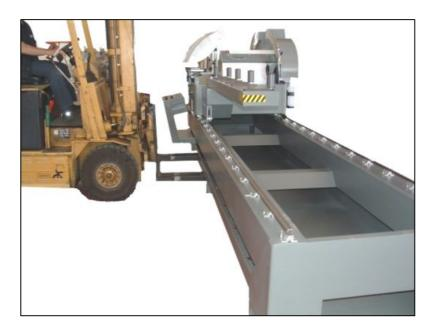
The machine rests on 6/8 adjustable feet, that allow the passing of the forklift.
