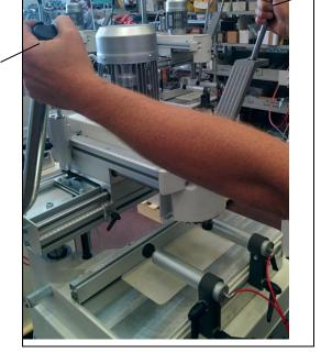
**a+b** Buttons for motor and lubrication start
