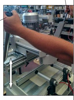
After starting the electric motor, lower the left lever (A) and consequently the head, proceeding to the drilling operation. Once finished reports the copy router at the initial position.
