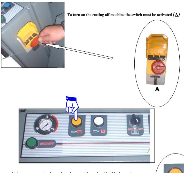
It is necessary to close the clamps otherwise the blade motor will not run. The PROTECTION COVER will close automatically when the blade will come out. To close the clamps the CLAMPS CLOSING BUTTON (B) must be pressed.
