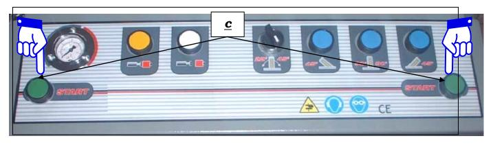
Once finished, releasing one of the buttons will cause the blade the return inside.
