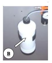
Periodically replace the cooling lubricant that is contained in the relevant tank (B). failure to observe this rule will invariably cause machining to be rougher and the mills to wear out more rapidly In the event that increased tool lubrication is required, use the regulator (C) of the exit of the cooling soupape which is placed inside of the machine near the blade.
