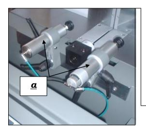
After the piece is locked with the clamps  $(\underline{a})$  and the motor started, press both (c) buttons. The blade will now move starting the cutting phase.
