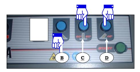
The machine has three fixed positions for the blade: 45°/90°/-45°.
