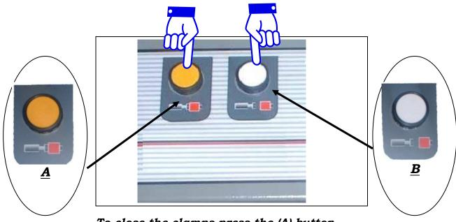
To close the clamps press the  $(\underline{A})$  button. Press  $(\underline{B})$  to open the clamps.
